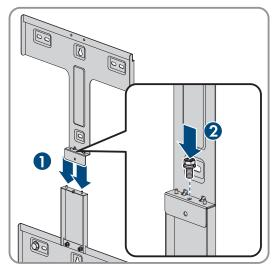
5. For battery modules directly above one another: align another wall mounting bracket on the connecting element and screw down with a supplied screw and washer assembly (TX20; torque 2.5 Nm).
