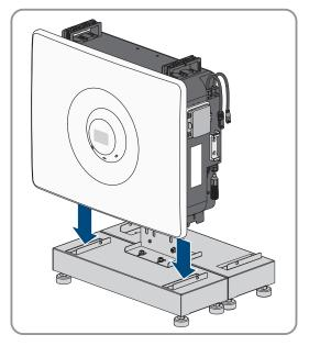
2. Attach the fixing brackets using 2 supplied screw and washer assemblies to each other (TX20; torque 2.5 Nm).
