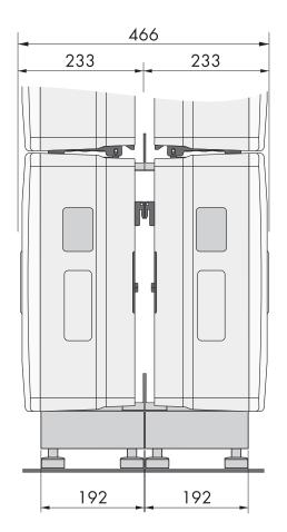
Figure 14: Position of the anchoring points (dimensions in mm)
