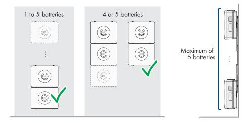
Figure 9: Wall mounting variants (recommended)
