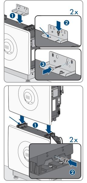
3. For 3 battery modules: now insert the fixing bracket; see above. Repeat the previous step for the third battery module.
