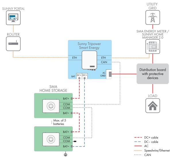
Figure 16: SMA Home Storage with 1 hybrid inverter (example)
