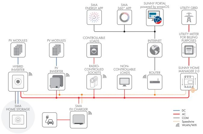
Figure 3: Design of the system (example)
