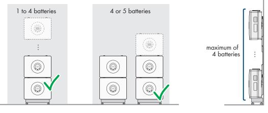
Figure 11: Mounting variants when mounting with base
