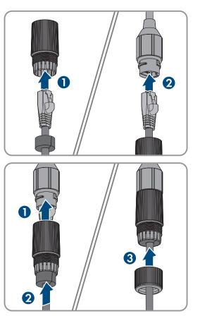
6. Secure the connection. To do this, firmly tighten the adapter and the swivel nut.
