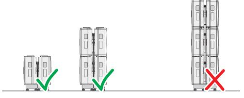
Figure 13: Mounting variants of the back-to-back
