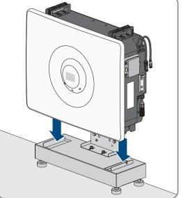
Attach battery module on the left and right to the base using supplied screw and washer assembly each (TX20; torque 2.5 Nm).
