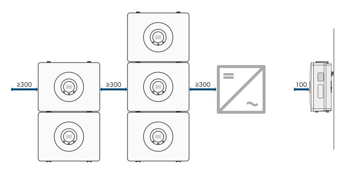
Figure 8: Recommended clearances (dimensions in mm)
