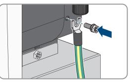
5. Connect the grounding cable to the external grounding point. The external grounding points of battery and inverter must have the same potential.
