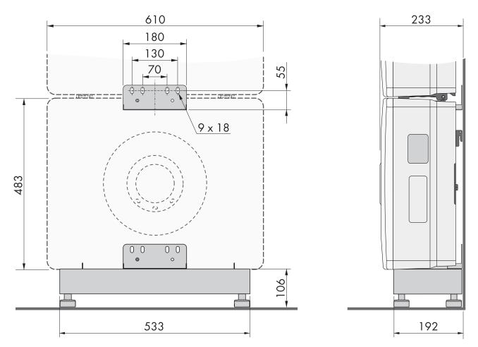
Figure 12: Position of the anchoring points (dimensions in mm)
