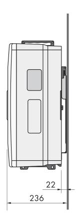
Figure 10: Position of the anchoring points (dimensions in mm)
