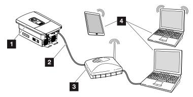
Fig. 7: Connecting inverter and computer
