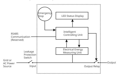
(Reserved) It is able to communicate with the inverters or smart meter via the RS485 communication port.
