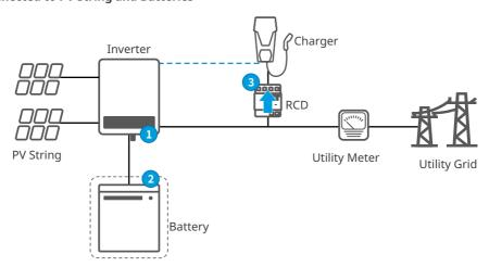
**Step 1** Turn on the AC and DC switches on the inverter side.
