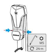
**Installing the Residual Current Device Distribution Board**
