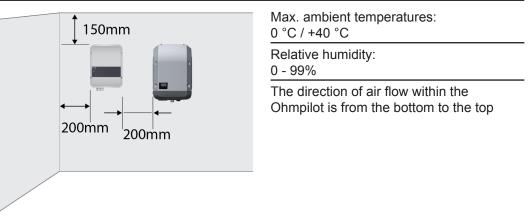
If the Ohmpilot is installed in an enclosed space, then forced-air ventilation must be provided to ensure adequate heat dissipation.
