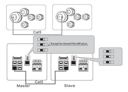
The connection diagram of three battery systems could be read below.
