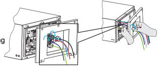
3. Fix the Operating Panel. To do this, insert the screws (M4x14) through the holes on them, using a Phillips screwdriver (PD2) and tighten it (torque: 2 Nm).
