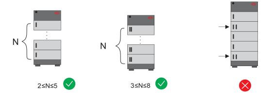
Up to maximum three battery systems could be connected in parallel. (This restriction does not apply for parallel connection with SMA Sunny Boy Storage 3.7-6.0. Please check the inverter operation manual on how to connect up to three batteries.)
