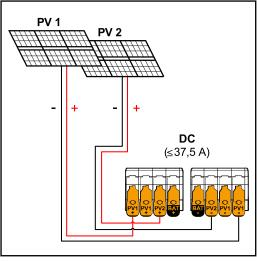
$PV 1 \le 18.75 \text{ A} / PV 2 \le 18.75 \text{ A}$
