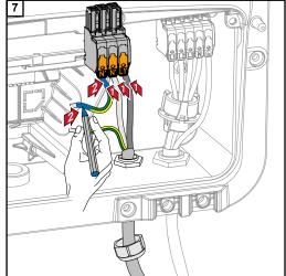
Strip the insulation of the single conductors by 12 mm.
