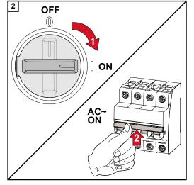
Set the DC disconnector to the "On" switch position. Switch on the automatic circuit breaker.
