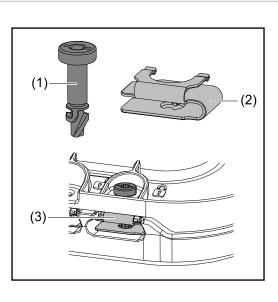
A quick-lock system (3) is used to mount the connection area cover and front cover. The system is opened and closed with a half-rotation  $(180^\circ)$  of the captive screw (1) into the quick-lock spring (2).
