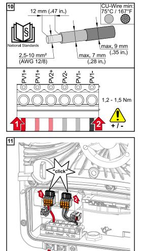
Strip the insulation on the single conductors by 12 mm and secure to the corresponding slot of the terminal on the PC board with a torque of 1.2 - 1.5 Nm.
