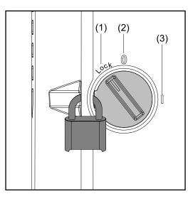
The DC disconnector has three switch settings:
