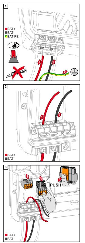
Manually push the BAT cables through the DC bushings.
