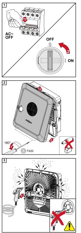
Switch off power to the inverter and wait for the specified time (2 minutes) until the capacitors have discharged and the fan has shut down. Turn the DC disconnector to the "Off" switch position.
