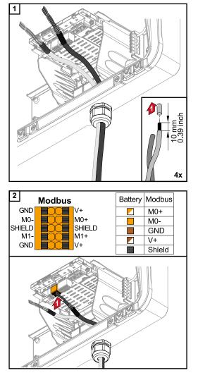
Strip 10 mm from the single conductors and mount the ferrules if necessary.
