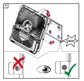
Clip the inverter into the mounting bracket from above. The connections must point downwards.
