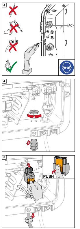
Drill out the optional cable guide with a step drill.
