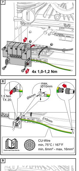
Insert the PC board into the inverter and secure with the four screws (TX20) supplied at a torque of 1.0 - 1.2 Nm.
