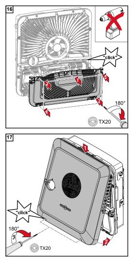
Place the cover on the connection area. Tighten the five screws by rotating them 180° to the right in the indicated order using a screwdriver (TX20).
