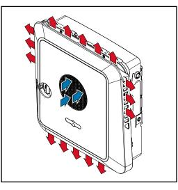
Ambient air is drawn in by the fan on the front side and blown out at the device sides. The even heat dissipation allows several inverters to be installed next to each other.
