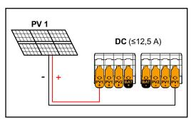
PV generator settings: PV 1: ON PV 2: OFF
