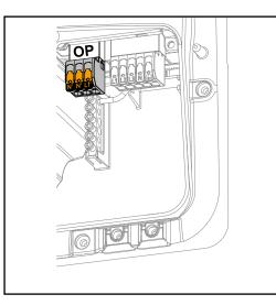
With the PV Point, in the event of a failure of the public grid, single-phase electrical devices can be connected to the Opportunity Power (OP) terminal and supplied with a maximum power of 3 kW, if enough power is available from the solar modules or an optional battery. In grid-connected operation, the OP terminal is not supplied with voltage, therefore the connected loads will not be supplied with power in this operating mode.
