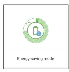
Energy saving mode is shown on the website of the inverter and in Solar.web by an "i" beside the battery symbol in the system overview. **BYD Battery-Box Premium** Fronius explicitly points out that the third-party batteries are not Fronius products. Fronius is not the manufacturer, distributor or retailer of these batteries. Fronius accepts no liability and offers no service or guarantees for these batteries.
