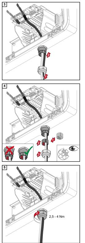
Guide the data cables first through the strain-relief device union nut and then through the housing opening.
