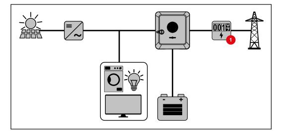
Operating mode -Inverter with battery and Ohmpilot
