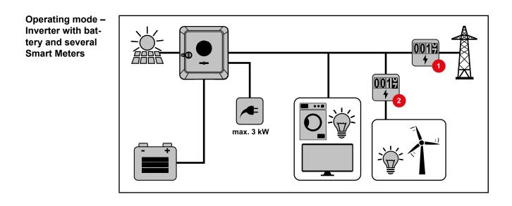
Operating mode inverter with battery, AC-coupled to another inverter
