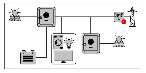
Energy flow dir-In the case of hybrid inverters, there are four different energy flow directions: ection of the in-
