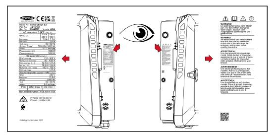
A 4-digit number (coded production date) is printed on the rating plate at the very bottom, from which the production date can be calculated.
